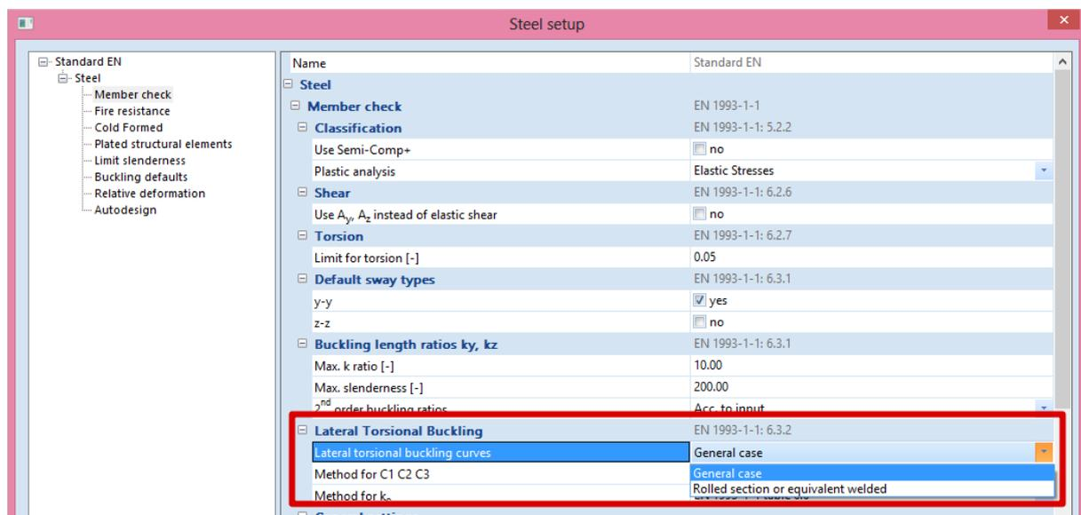
With this option the reduction factor for Lateral Torsional buckling is calculated a bit differently:
